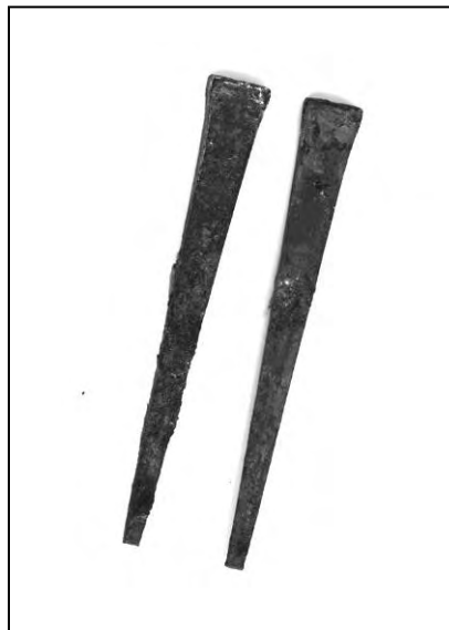
Fig. C-021. Flooring nail at pantry, detail showing slightly beveled and flared heads. (GWWO photo, 2005)
