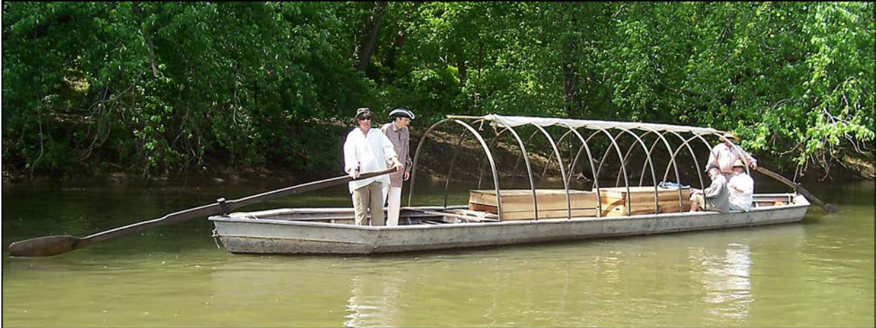
Replica of a James River tobacco batteau. Note the sweeps at both ends used to steer the boat. (D. Guzy)
