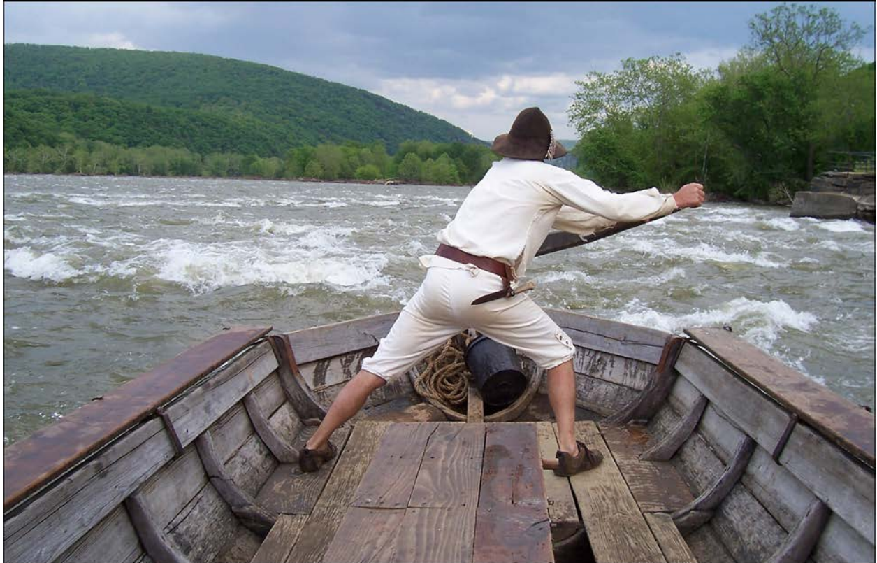
Boatman using the front sweep to steer through white water in a replica batteau—looking downstream. (D. Guzy)
